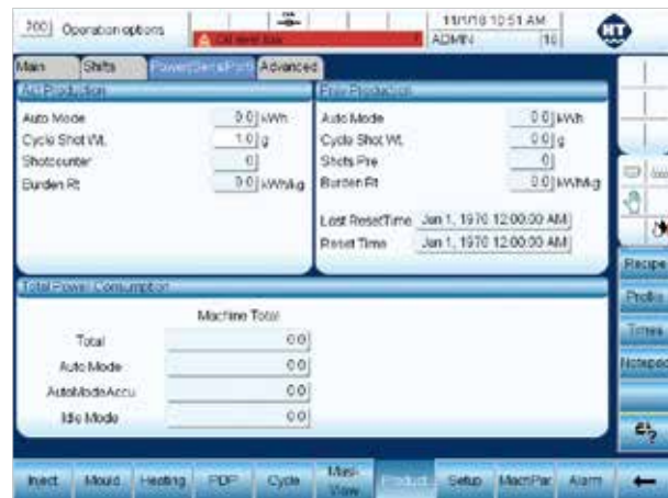
Energy control and monitoring over the production process and equipment operation status
