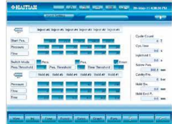
Injection screen: 6-stage injection control
