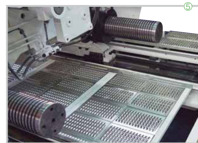
Figure ③ Reverse mounted ejection plate with the flexibility for optional longer strokes.
