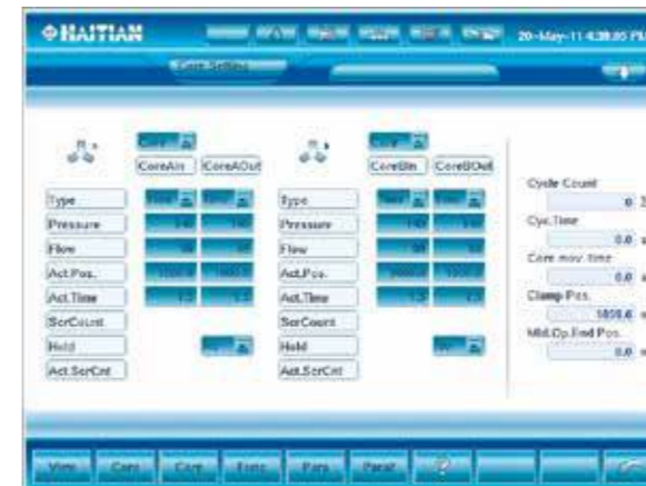
Core screen: Flow and pressure controllable
