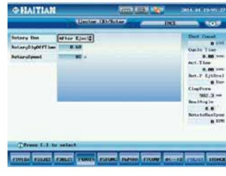
The control system of the servo hydraulic turntable is equipped with a rotating encoder, which provides immediate feedback on the turntable location. By changing the degree of opening of the turntable's proportional direction valve as well as the system's pressure and flow, the closed loop control is established.
