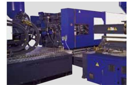
**Flexible side injection unit positioning**
