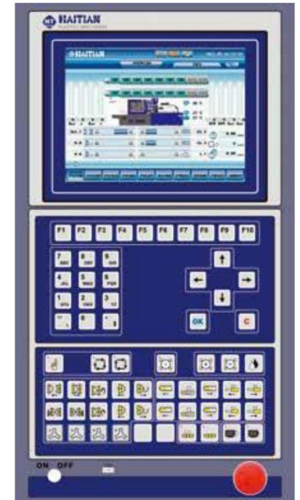
Control system especially for the multi component injection molding machines, with two CPU for the parallel processing of data. The newest, easy to use computer control system, with a faster response cycle.
