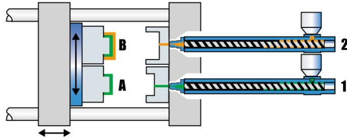
Injection Unit 1 and 2 work in parallel. Ejection (part A and part B), Then the table rotates 180°. After the mold is closed, Both part A and part B injection will be finished at the same time, then the mold opens. The process always repeats again as above.
